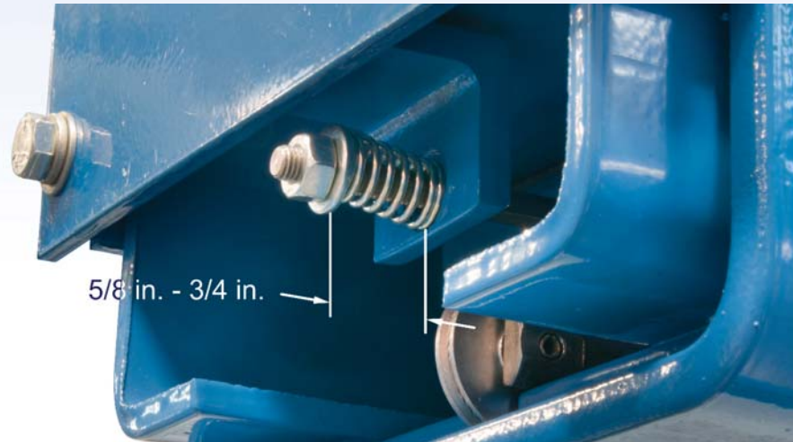
Figure 11 Extend Cable Spring Adjustment
