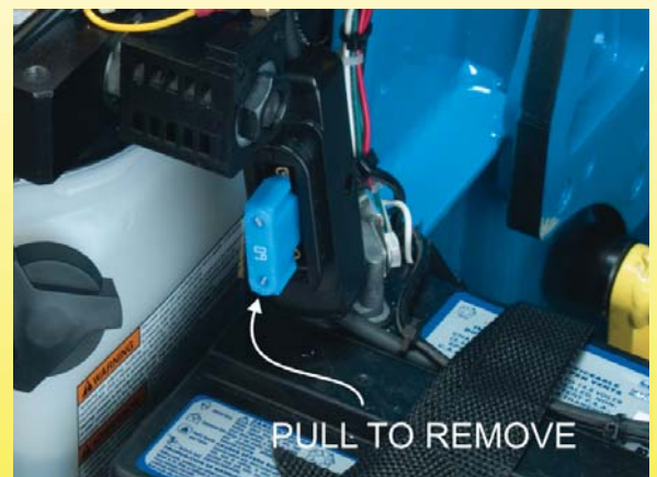
Figure 27 Main Power Fuse
