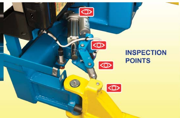
Figure 33 Outrigger Inspection Points
