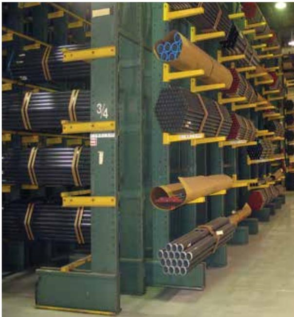
Cantilever rack allows storage shelves without front obstructions, with solid decking covering the entire length of the rack row. The result is a system where loads of varying lengths can be placed anywhere along the entire storage shelf.
