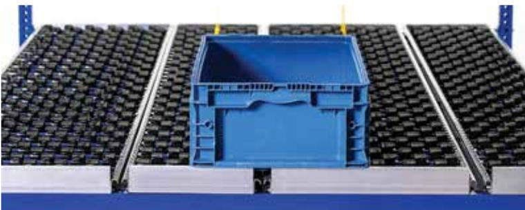
Left: allows loads to overlap lanes and still easily flow for versatile storage
