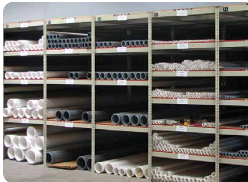
Above: rivet shelving can store long, heavy loads such as pipe and tubes
