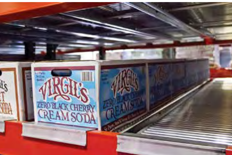
Above: Full cases presented for picking in a flow rack system.
