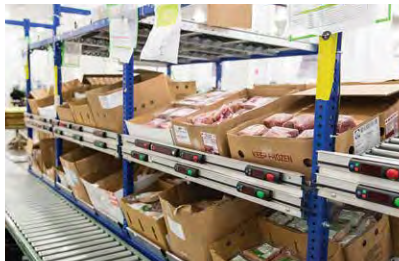
Above: tilted shelves to allow easy access for each-pick operations.
