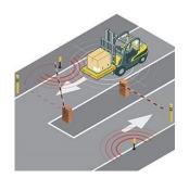
Vehicle access systems: gates are automated through use of a ZoneSafe antenna system that creates a detection zone around the gate. Transponder tags signal the antenna to open the gate as they approach.
