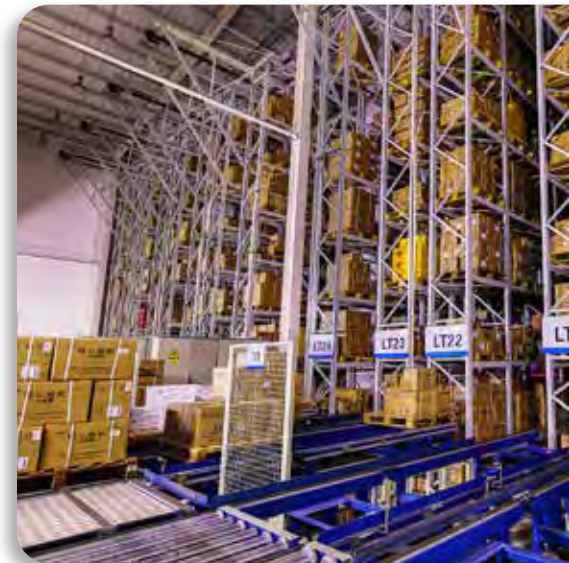
AS/RS systems demand high capital investment and require specialized integrations and maintenance, but reduce labor usage and increase safety. They're ideal for space-pressed environments where speed, accuracy and throughput are critical. They are the most complex, but also the most automated of pallet storage/retrieval solutions.
