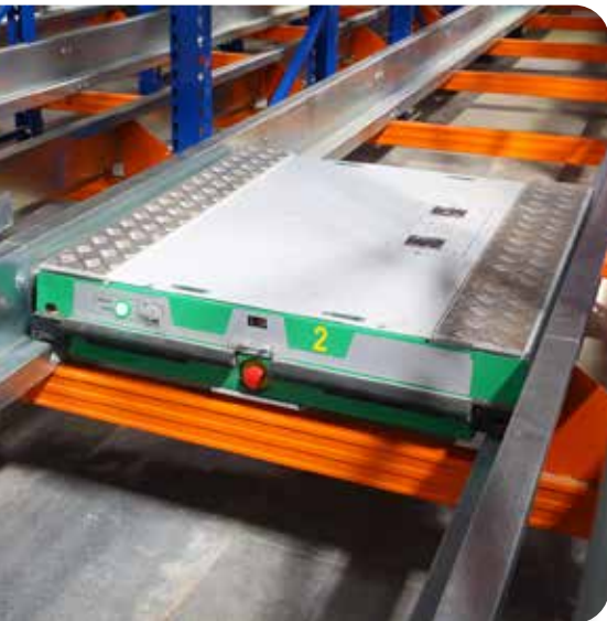
Pallet shuttles are a semi-automated solution that strikes a balance between AS/RS and manual forklift/racking. They improve high storage density by eliminating fixed aisles. While not as fast or precise as a full AS/RS, they improve retrieval speeds and reduce labor needs compared to conventional methods.
