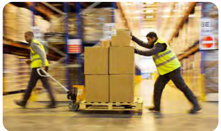
Above: for heavier loads (above 50 pounds push force) use powered pallet jacks where possible. Two people can transport the same load in cases where loads are extremely heavy.
