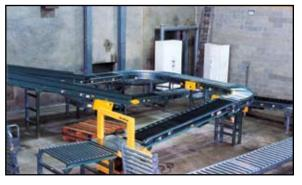
ing conveyors from the two scale lines into the sortation mezzanine feed conveyors.
