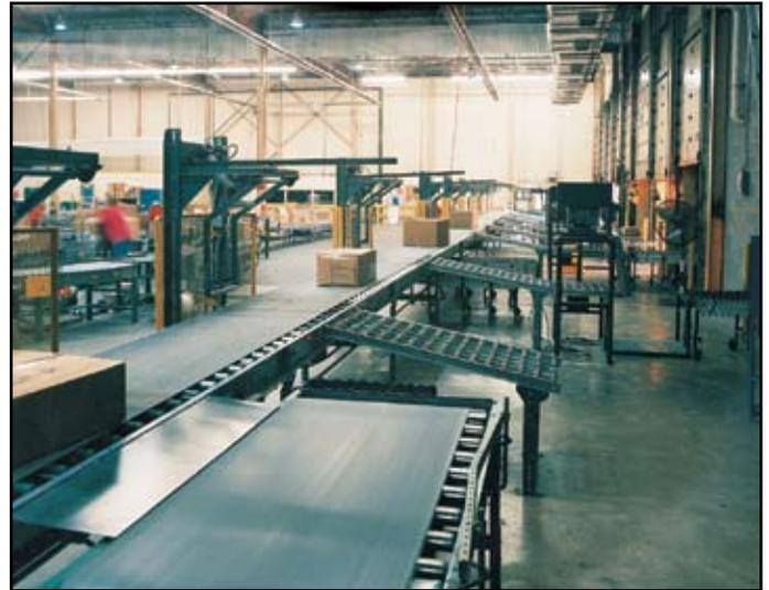
loop of minimum-pressure accumulation conveyor. The cartons then travel through a scanning location where their dock destination is determined. The information is transferred to the system’s primary logic controller which activates an overhead pusher at the appropriate dock location. Cartons flow onto an extendible conveyor that transports them into trailers for loading.
