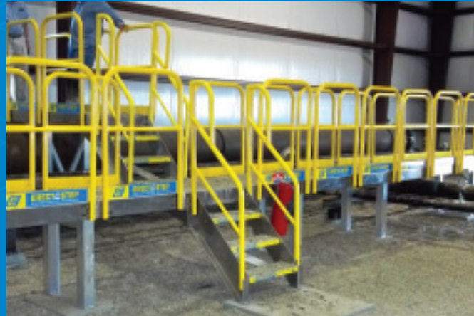
Each support height has a matching stair.
