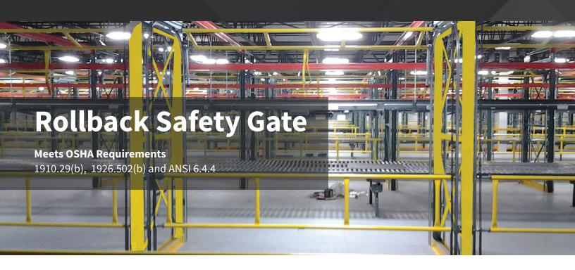
Protect workers on elevated access points for material transfer. The gate is easy-to-use and install and protects without hindering productivity. A two-gate system means one gate is always closed and OSHA compliant fall protection is in place.
