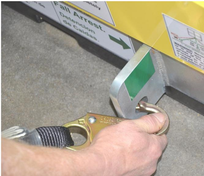
Connect to the Round Loop only for Fall Restraint.
