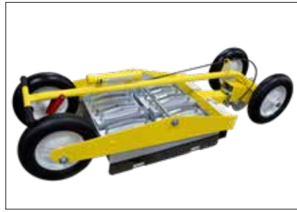
Press handle release and lower weights into working position.
