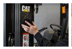
STEP 1: Wash Mast Wash any oil/grease from mast
