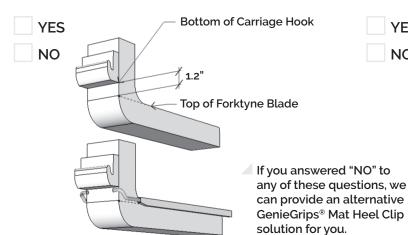
**TYPE B** - is there **0.8 inches clearance** between the side of the Carriage Hook and the side of the Forktyne Blade?
