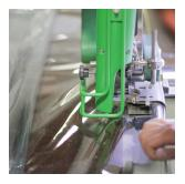
Goff's Clean Curtain Walls utilize heat-seal technology to fuse edges and seams, eliminating potential contamination. This also provides a clean and finished edge.
