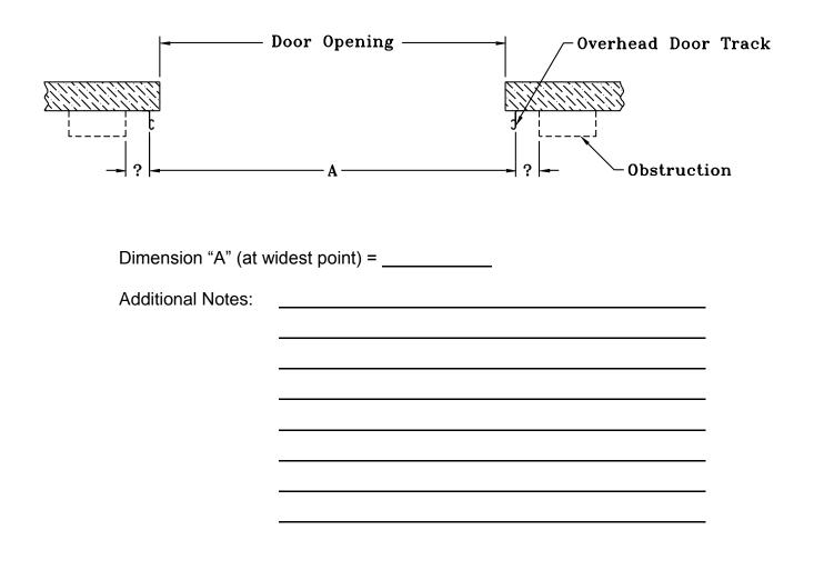
Carefully Measure the "setback" of the existing Overhead Door track at the floor level (Dimension "B" in the following diagram) and at a location 9" (nine inches) for Gravity Doors OR 14" (fourteen inches) for G2 Doors above the door opening (Dimension "C" in the following diagram). Also note the dimensions and locations of any potential obstructions (control boxes, bollards, etc..).
