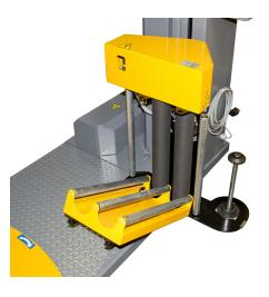
**Digitally controlled power film pre-stretch** (250% standard) for dynamically controlled film efficiency and improved load containment, both lowering consumable cost and keeping your product safe and secure
