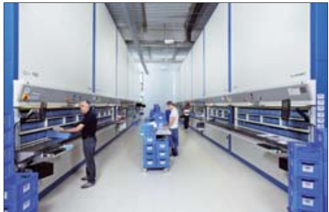
Small parts are picked quickly and efficiently from 12 Hänel Rotomat® storage carousels
