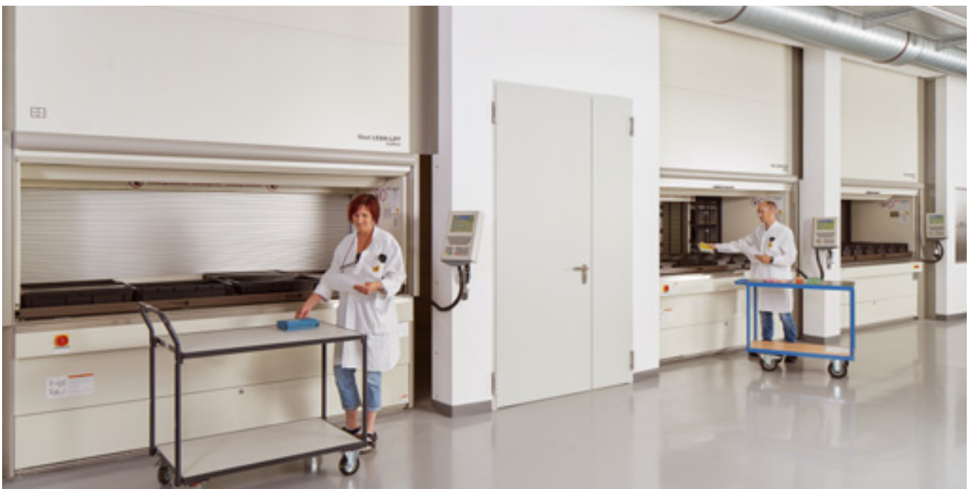
The first of three Hänel Lean-Lifts® on the ground floor also has an additional access point on the top floor to ensure fast provisioning of electronic components
