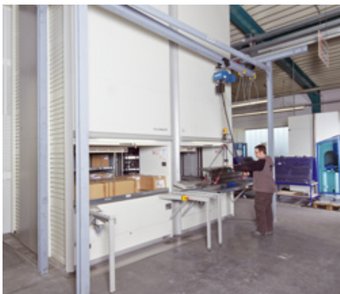
Folding rails bear the weight of extremely heavy items, thus making retrieval or replenishment much easier
