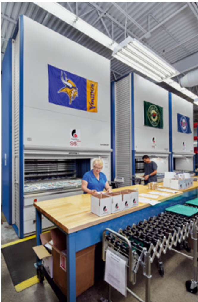
High pick rates thanks to parallel operations using several Hänel Lean-Lift® high-speed systems
