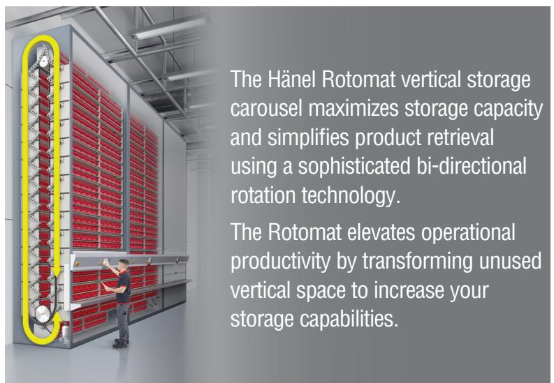
The Hänel Rotomat vertical storage carousel maximizes storage capacity and simplifies product retrieval using a sophisticated bi-directional rotation technology.
