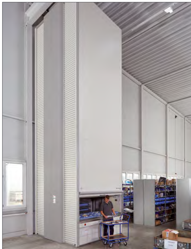
This Hänel Lean-Lift® has a height of more than nine meters to provide a huge amount of storage capacity and thus save considerable floor space
