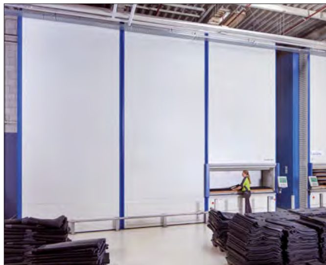
Items stored in the Hänel Multi-Space® are transported with maximum speed because the extractor moves horizontally and vertically
