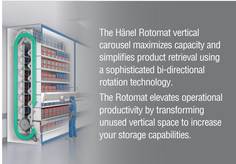
The Hänel Rotomat vertical carousel maximizes capacity and simplifies product retrieval using a sophisticated bi-directional rotation technology.
