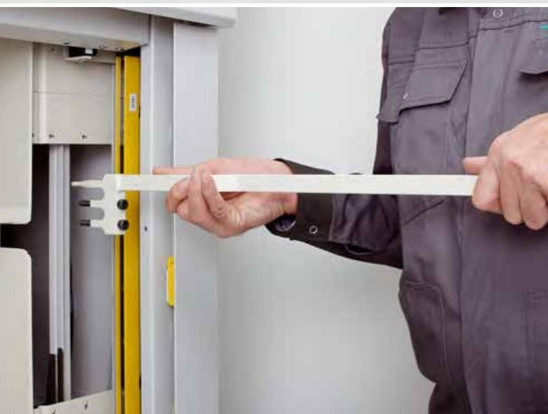
The Hänel arresting device for safe maintenance of the Hänel Rotomat® storage carousel
