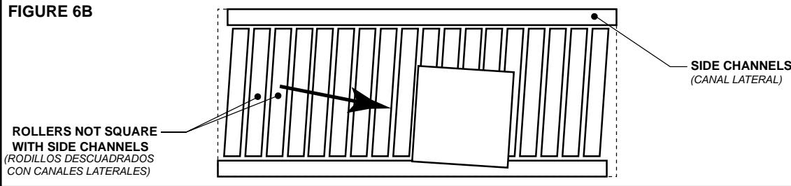
"Racked" conveyor sections will cause package to travel toward side of conveyor.
