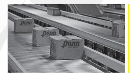
The model ABEZ is a belt driven, live roller conveyor designed for applications that require accumulation of product without a build-up of line pressure and comes standard with a centralized drive capable of conveying 150 pounds per linear foot.
