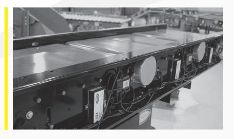
The model 190-RBE24EZ is a direct drive conveyor equipped with a series of Hytrol's E24™ 24-volt DC motors to drive the rollers. The 190-RBE24EZ is an automatic tracking and tension belted conveyor. Because of this, there are no manual tracking or tension adjustments needed.
