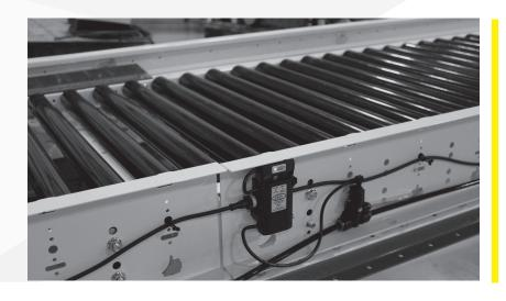
The model 190-GEZ is a gravity conveyor that is ideal for declines and maintaining control of product. It is equipped with EZLogic® for accumulation.
