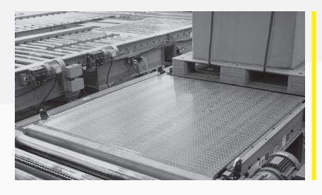
The model PLEZD is a plastic belt conveyor designed to handle footed pallets, slip sheets, unitized loads—items normally non-conveyable on roller conveyor. The PLEZD provides zero-back pressure accumulation, reducing the possibility of product damage and can handle up to 2,000 pounds per zone.
