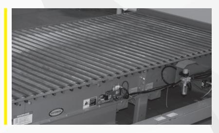
The model 25-LREZ is a heavy-duty belt driven live roller conveyor designed for use where zero-pressure accumulation, low elevation and close roller centers are required. The 25-LREZ is capable of conveying 1,000 pounds per linear foot.
