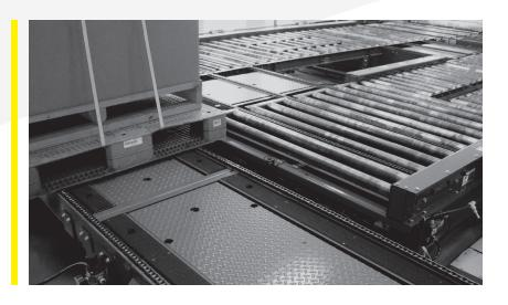
Model DCEZ-60 and DCEZ-82 are drag chain conveyors designed for pallets. With an EZLogic® accumulation module, pallets are accumulated with zero-back pressure reducing the possibility of collision that may result in product damage. Both are capable of conveying 12,000 pounds at 30 FPM.
