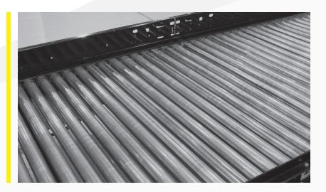
The model 199-PVEZD is a Poly-V Belt driven live roller conveyor designed for zero-pressure accumulation of product. This conveyor is designed to handle cartons or pallets. The Model 25-PVEZD is designed to handle heavy pallets, drums, containers, etc.—capable of conveying 250 pounds per linear foot. Products may be accumulated in zones and released upon request.
