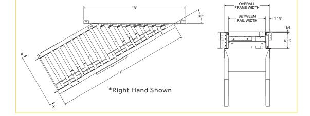
190-E24EZSS 24VDC 45° Live Roller Accumulating Straight Spur Conveyo
