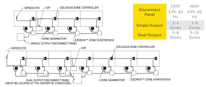
Note: Infeed Wake-Up Eye used only on terminating infeed end of conveyor. Not used when connecting to upstream EZLogic® conveyor through power supply isolation cable.
