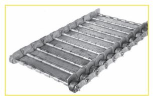
Metal Piano Hinge belt provides continuous reliable service. Construction is heavy-duty with perforated apron plates and solid steel, heat-treated rollers.
