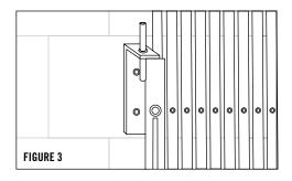
**4)** Extend and retract gate to its stops to work out stiffness, then fully extend gate across opening. Align padlock holes and position the locking bar on door frame or wall. Mark and drill pilot holes. Secure with 5/16" x 2" lag bolts. (See Figure 4)
