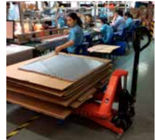
The manual Thork Lift needs very low power for the pump function and has foot protection and neutral position.
