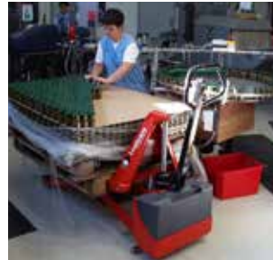
The emergency stop is centrally placed on the electric Thork Lift. The forks stop quickly and precisely.
