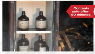
Contents remain intact after a 90-minute burn test.
