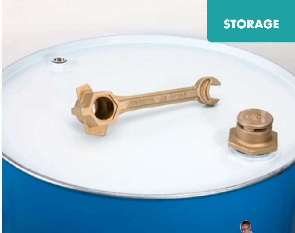
Above: Vent on a vertically stored drum provides automatic relief of both pressure and vacuum. A brass nonsparking drum wrench safely opens tight bungs.
