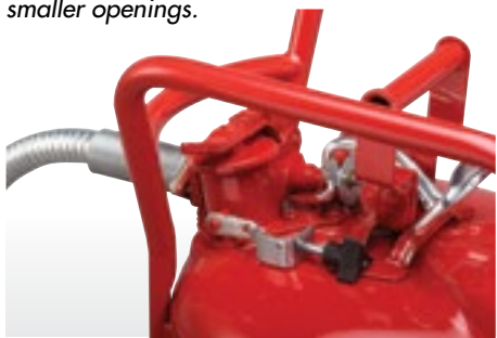
Type II D.O.T. Safety Can Two openings: top opening with lift lever for filling, and a second one with flexible metal hose attached for accurate, plug-free dispensing into smaller openings. Additional safety features include roll-bar construction and a fusible-link protected hold-down bracket for protection during over-the-road transport.
