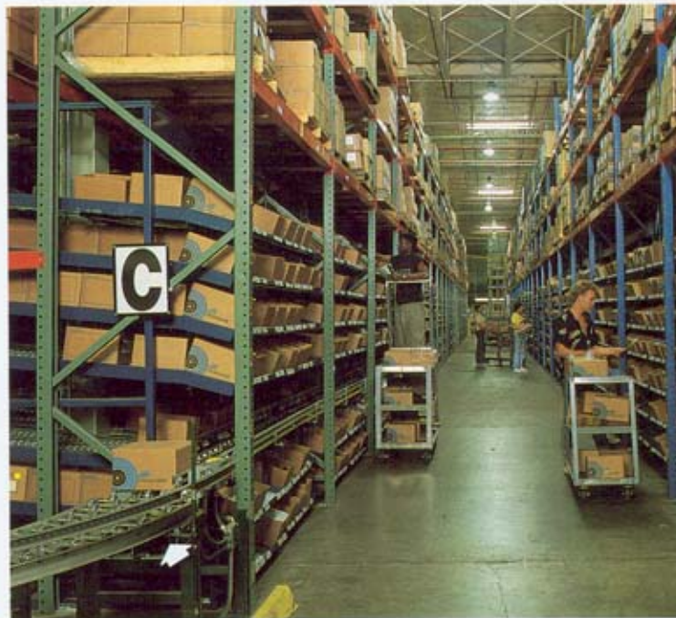
Keneco systems with knuckled shelves speed picking. System at right equipped with optional built-in takeaway conveyor (see arrow).
