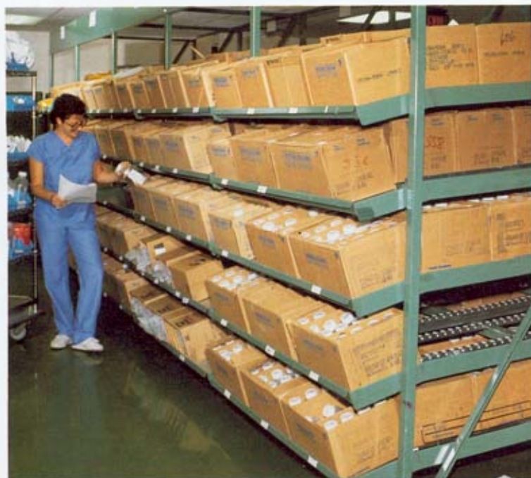
Keneco systems with knuckled shelves speed picking. System at right equipped with optional built-in takeaway conveyor (see arrow).
