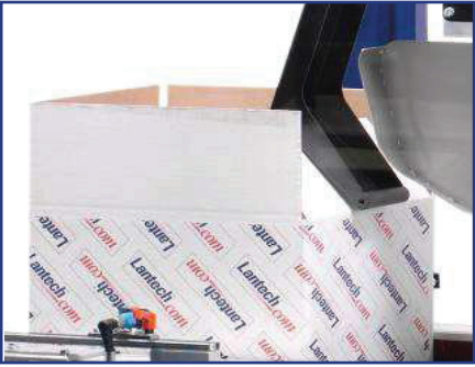
PRE FOLDING THE SHORT FLAP Wide and thin corrugated cases can be handled because of pre folding the first short flap. This helps avoiding packaging damage and improves the reliability of your packaging process.
