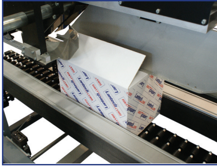
TOP CLOSING The side belts transport the case underneath special designed stainless steel curves. Due to the movement the long flaps close perfectly.
