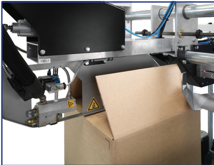
HOTMELT CLOSING VERSION During the folding process hotmelt is applied on the two inner flaps. Directly after this the outer flaps are folded and glued to the inner flaps.
