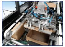
Adjustable Forming Unit The long sides of the incoming tray are glued during infeed and are positioned and held in place by 2 brackets for accurate lid applica-tion. The lid is moved to the tray and the 4 flaps are folded 90° and glued on the tray.
