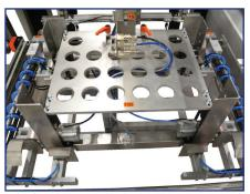
Adjustable Forming Unit The folding unit is adjustable in length and width and can be adjusted to the correct tray size. The adjustments are done by hand wheels and can easily be read from counters and scales.
