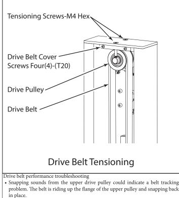
Cracking or snapping noises from the lower drive pulley is most likely a tensioning or loose belt condition. Under load this condition could be worse and the unit may not lift a load.
