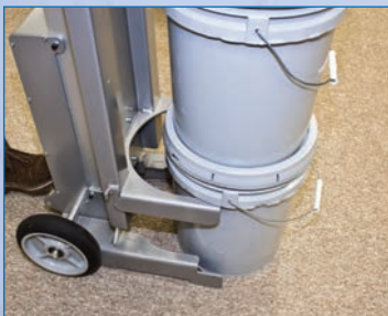
Lifting yoke holds pails in place.
