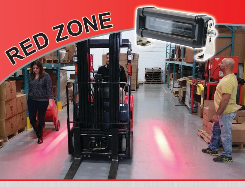
40% of all forklift accidents involve a pedestrian. Ensure pedestrians stay a safe distance away from the lift truck with the Red-Zone LED Warning Light. The Red-Zone emits a red beam on the floor to keep pedestrians away preventing foot injury or collisions from rear end swing.
