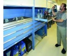
Storage Wall sections with tambour doors, roll-out trays with FOD cut-outs, drawers and open storage space at bottom.
