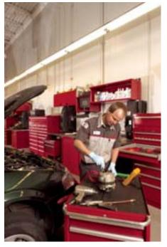
Each technician's mobile cabinet can bring tools and a worksurface to the car being serviced.
