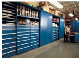
The Storage Wall System enables the New York Daily News to store oversized items such as motors, gears and drive shafts on shelves, while keeping smaller items such as drill bits and hand tools in highly organized, adjacent modular drawers. Lockable sliding doors keep contents safe and secure.
