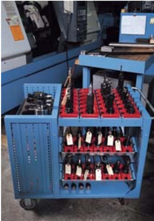
*Lista CNC tool transporters are used to safely deliver tools directly to the work area at Continental Machines, a leading machine tool and hydraulic component manufacturing company.*
