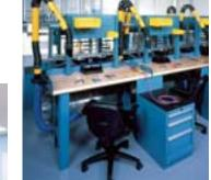
Lista's custom solution for this manufacturer of silver giftware included workbenches with cut-outs for particle recovery systems and speciallyconfigured companion drawer cabinets.
