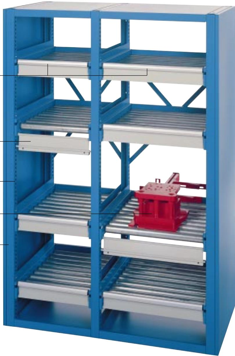
*Designed to bring additional heavy-duty storage and convenience to Lista's modular Storage Wall system, the Storage Wall Roller Shelf is constructed of standard conveyor rollers, a front security gate and backstop. This unique solution allows items that weigh as much as 770 lbs. to easily glide into and out of the Storage Wall. Ideal for the storage of dies, molds and other heavy equipment and parts, the Roller Shelf is safe, ergonomic, and entirely unique.*
