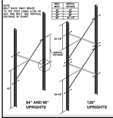
STEP 4A ASSEMBLY USED FOR BACK TO BACK **SECTIONS ONLY**
