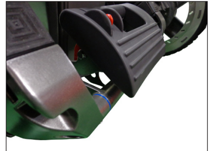
Not Locked Properly
