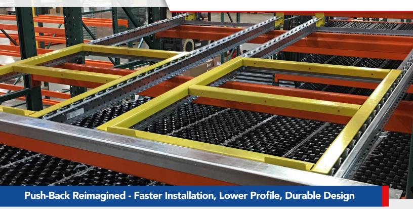
Who better than the gravity flow experts to reinvent LIFO storage? Mallard's push-back cart system pairs steel skate wheel rails with custom carts to deliver superior results. Wheeled rails are more durable than carts with individual wheels saving installation and maintenance costs.
