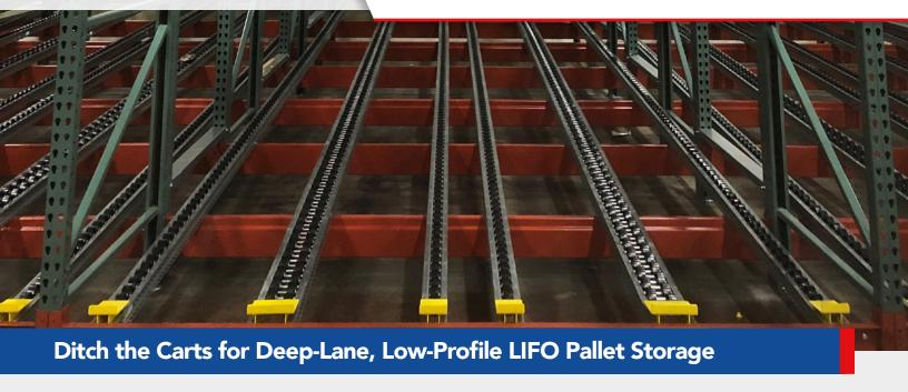
Push-back flow rack relies on gravity flow tracks and eliminates the need for carts. Your push-back flow rack system accommodates pallets of varying sizes and provides very low-profile storage no matter how deep the lane. Single aisle access creates a consolidated LIFO footprint.
